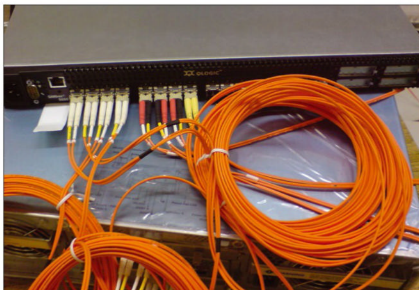
Figure 1: Fibre Channel hardware such as this switch from QLogic has long been standard in the data center. Today, FC is increasingly giving way to Ethernet. © Wikipedia/Melee
