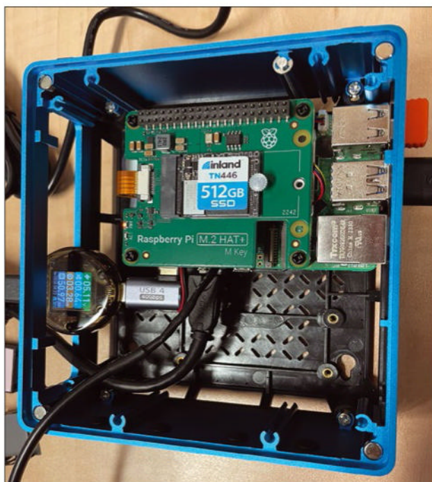
Figure 3: Installing the M.2 HAT+ and NVMe drive altered the idle power draw a hardly noticeable 0.2W.
