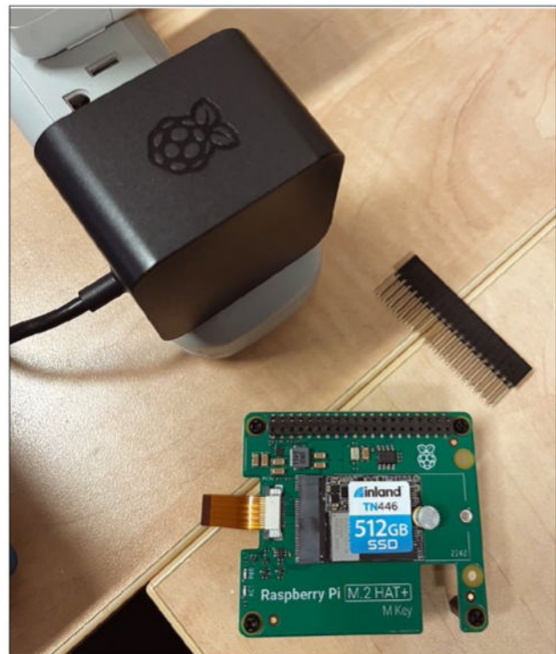
Figure 2: The standoffs and GPIO extension included with the M.2 HAT+ permit installing clear of the CPU fan.
